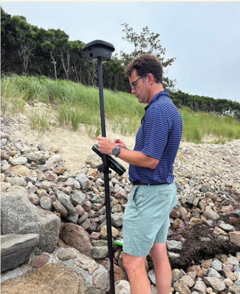
Trey Ruthven of Sustainable Coastal Solutions measuring the contour of the harbor bank.
